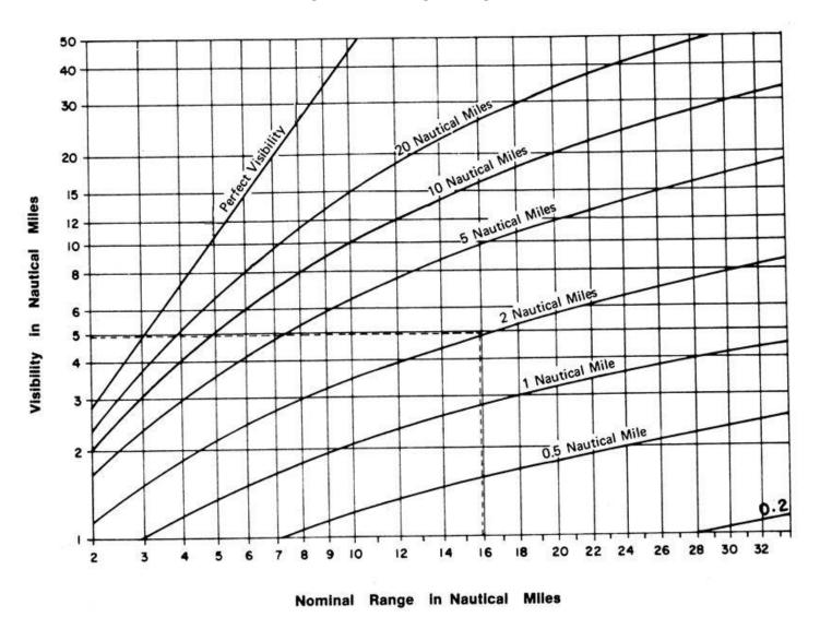
The light list in column 7 gives the nominal range of each lightstation optic where there is sufficient light to be seen 2 nautical miles or more when the meteorological visibility is 10 nautical miles.
